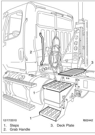
Fig. 2.6, Back-of-Cab Access Supports (typical)
