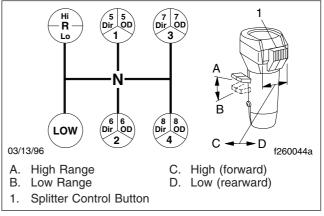
Fig. 13.1, Eaton Fuller 13-Speed Transmission Shift Pattern
