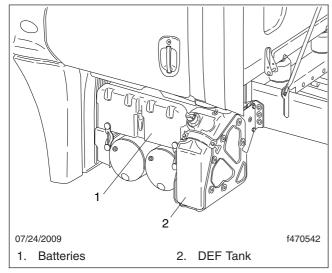
Fig. 11.8, DEF Tank Located Behind the Battery Box
