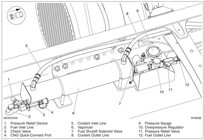
Fig. 21.11, LNG Vaporizer Assembly
