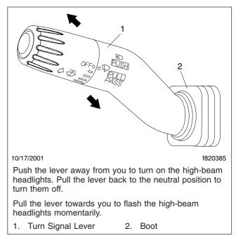
Fig. 5.7, High-Beam Headlight Operation
