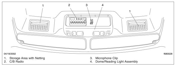
Fig. 5.4, Overhead Control Panel
