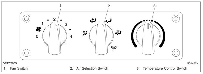
Fig. 7.1, Climate Control Panel Without Air Conditioning
