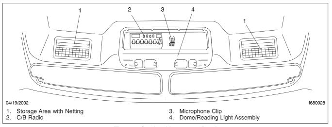
Fig. 4.14, Overhead Instrument Panel
