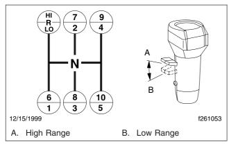
Fig. 13.3, Eaton Fuller 10-Speed Transmission Shift Patterns
