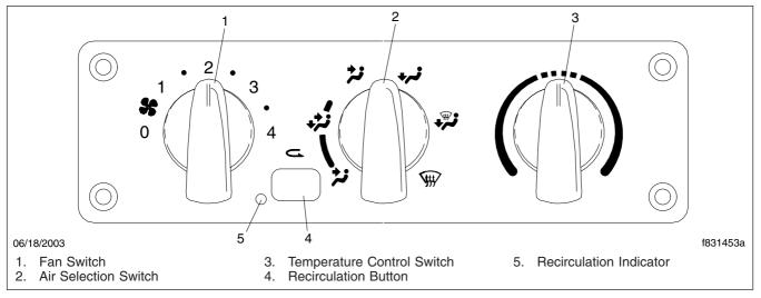
Fig. 7.2, Climate Control Panel With Air Conditioning
