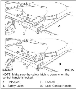
Fig. 17.2, Fontaine Locking Mechanism
