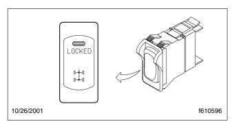
Fig. 5.18, Differential Lock on Single Drive Axle
