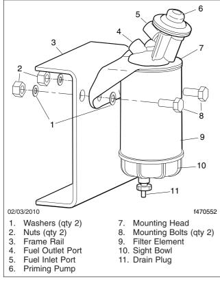
Fig. 21.12, Alliance Fuel/Water Separator Assembly and Installation
