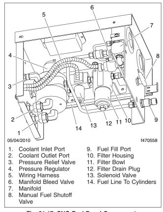
Fig. 21.17, CNG Fuel Panel Components
