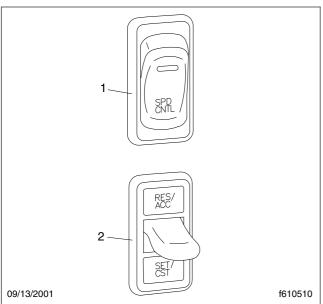
To turn cruise control on, press the upper half of the On/Off switch. To turn cruise control off, press the lower half of the On/Off switch.
