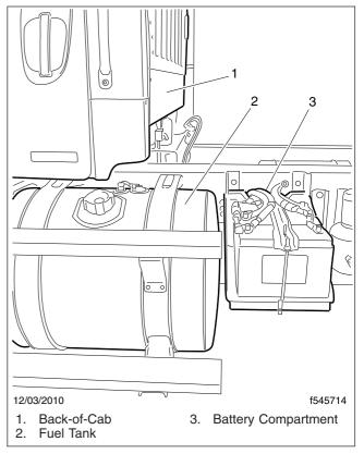
Fig. 3.4, Standard Battery Compartment Location
