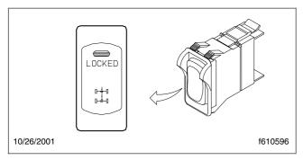
Fig. 15.1, Differential Lock on Single Drive Axle
