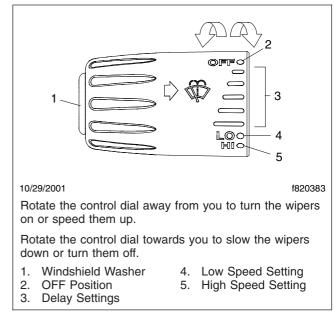
Fig. 5.13, Windshield Wiper/Washer Controls
