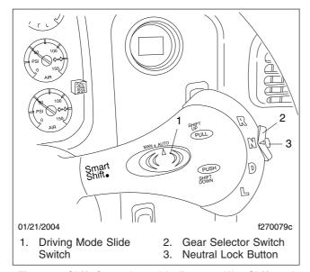
Fig. 14.2, Shift Controls and Indicators, UltraShift and **AutoShift Transmissions**
