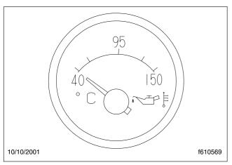
Fig. 4.10, Engine Oil Temperature Gauge
