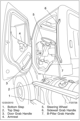
Fig. 2.4, Cab Access System, Driver's Side
