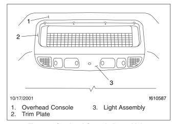
Fig. 5.11, Overhead Console Dome Lights
