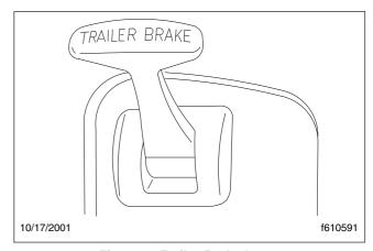
Fig. 5.31, Trailer Brake Lever
