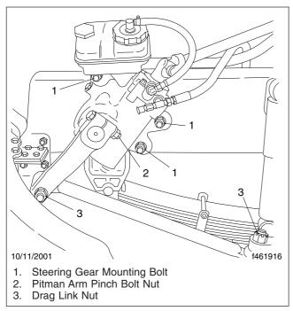
Fig. 21.14, Steering Gear Fasteners
