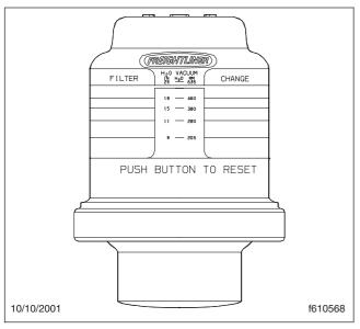
Fig. 4.5, Air Intake Restriction Indicator
