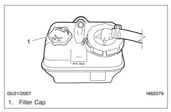
Fig. 21.6, Power Steering Fluid Reservoir
