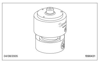
Fig. 4.6, Manual-Reset Air Restriction Indicator, Go/ No-Go
