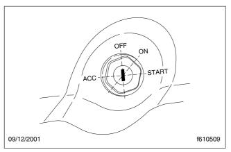
Fig. 19.7, Ignition Switch Positions
