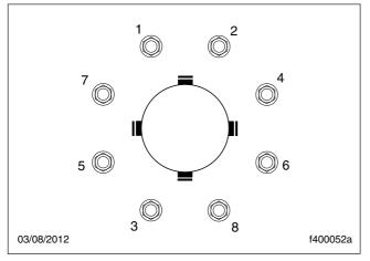
Fig. 21.5, Tightening Pattern, 8-Hole Wheels
