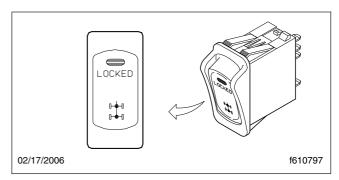
Fig. 15.2, Differential Lock on Both Axles
