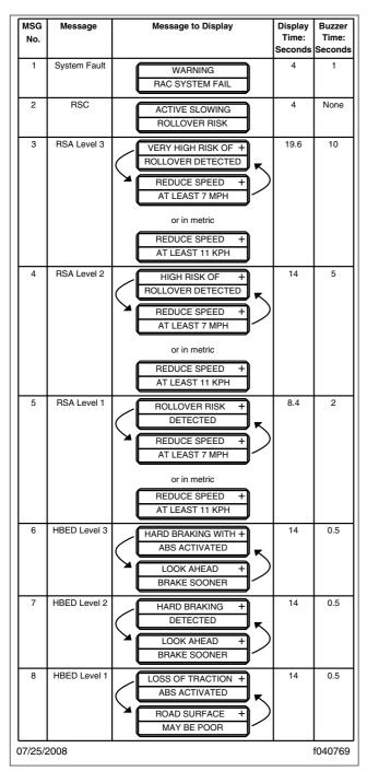
Fig. 12.5, Roll Stability and Hard-Braking Warnings
