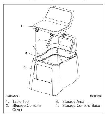
Fig. 8.1, Center Storage Console (with writing surface)
