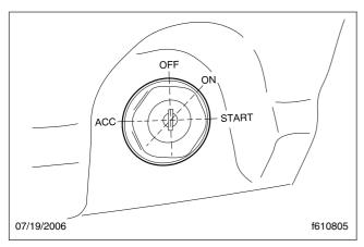
Fig. 5.1, Ignition Switch Positions
