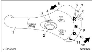
To upshift manually, pull the lever back (towards the driver). To downshift manually, push the lever forward (away from the driver).
