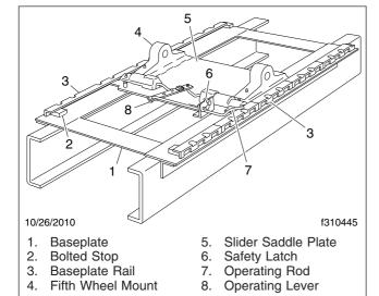
Fig. 17.13, Sliding Fifth Wheel Manual Release, Holland Simplex
