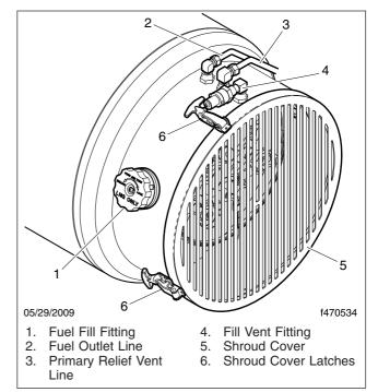
Fig. 19.2, LNG Fuel Tank
