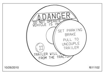
Fig. 17.10, Air-Actuated Kingpin Release Valve
