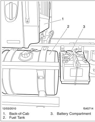
Fig. 21.15, Standard Battery Compartment Location
