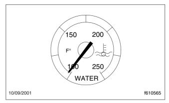
Fig. 4.7, Coolant Temperature Gauge
