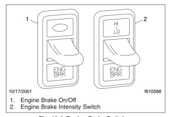
Fig. 10.4, Engine Brake Switches
