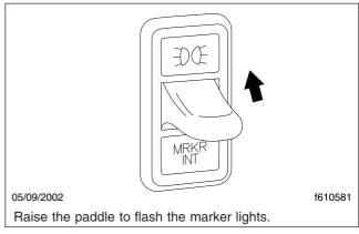
Fig. 5.8, Marker Light Interrupt Switch
