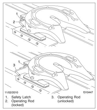
Fig. 17.3, Holland Simplex SE Locking Mechanism
