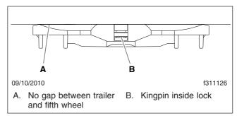
Fig. 17.6, Coupling Inspection
