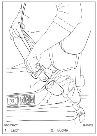
Fig. 6.9, Three-Point Seat Belt Operation
