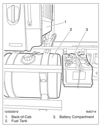
Fig. 24.4, Standard Battery Compartment Location
