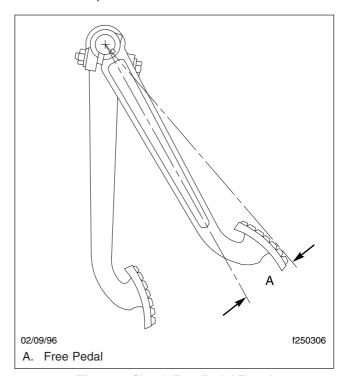
Fig. 13.4, Clutch Free Pedal Travel
