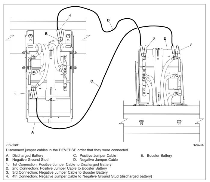
Fig. 24.6, Jumper Connections
