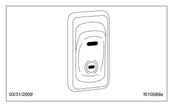
Fig. 5.25, Exhaust Brake Switch
