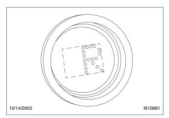
Fig. 14.6, Gear Indicator: Reverse Low Gear
