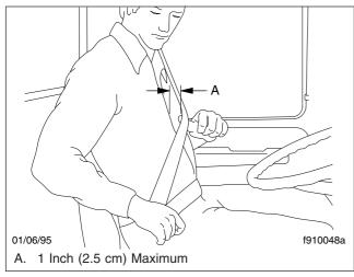
Fig. 6.11, Adjusting Shoulder Harness Clearance, Komfort Latch
