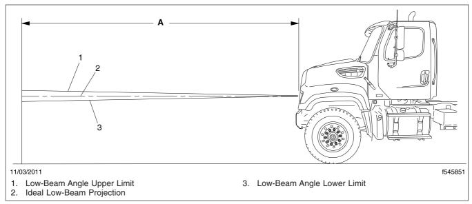
Fig. 23.2, Vertical Low-Beam Headlight Variation Limits
