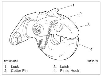
Fig. 18.1, Holland PH-760 Trailer Coupling
