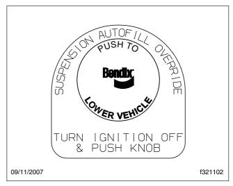
Fig. 5.32, Suspension Autofill Override Valve
