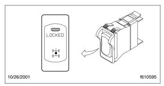
Fig. 15.4, Interaxle Lock Switch
