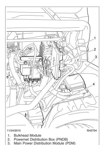
Fig. 21.7, Visible Engine Wiring
