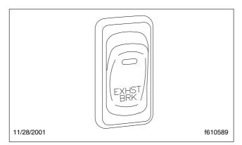
Fig. 5.24, Exhaust Brake Switch
