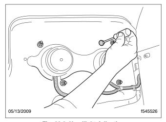
Fig. 23.3, Headlight Adjusting
