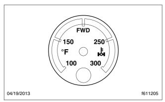
Fig. 4.8, Forward-Rear Drive Axle Oil Temperature Gauge
