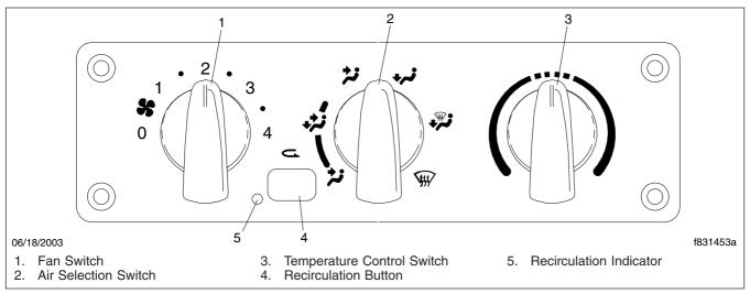
Fig. 5.35, Climate Control Panel With Air Conditioning
