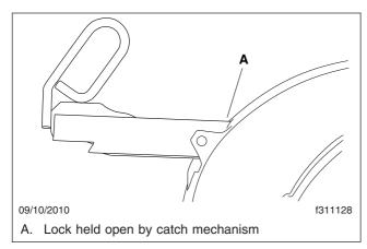
Fig. 17.7, Jost Release Handle Unlocked
