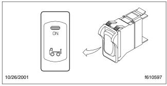
Fig. 17.1, Air-Suspension Dump Valve
