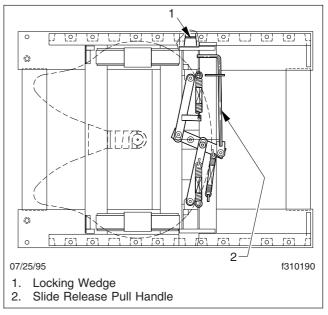
Fig. 17.11, Manual Release Sliding Fifth Wheel, Fontaine
