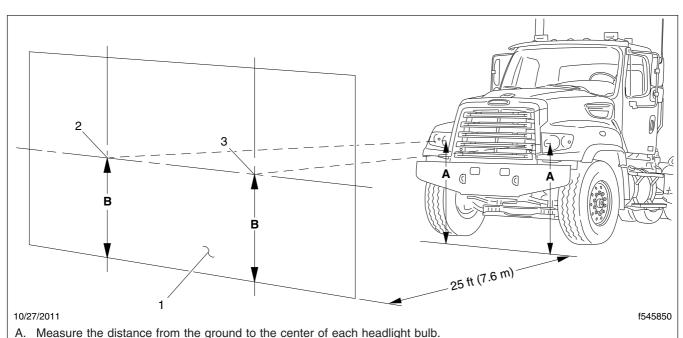
Fig. 23.1, Headlight Aiming Screen/Wall
