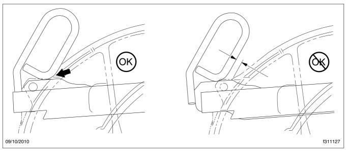
Fig. 17.8, Jost Release Handle Locked
