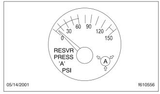
Fig. 4.12, Air Pressure Gauge (reservoir A shown)
