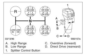
Fig. 13.2, Eaton Fuller 18-Speed Transmission Shift Pattern
