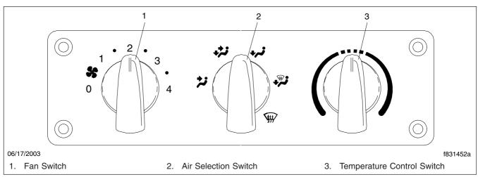
Fig. 5.34, Climate Control Panel Without Air Conditioning
