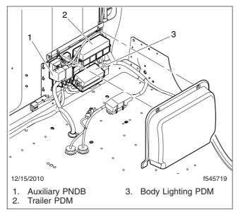
Fig. 3.2, Auxiliary Power Distribution Module
