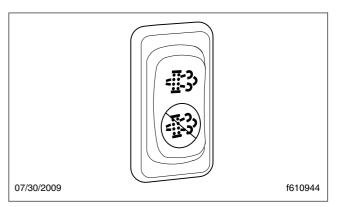
Fig. 11.2, Regen Request/Inhibit Switch
