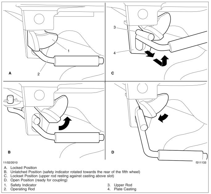
Fig. 17.9, Holland Kingpin Locking Mechanism
