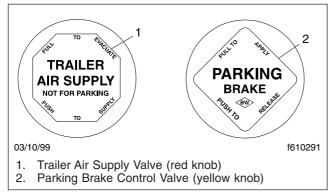
Fig. 5.30, Brake Valve Control Knobs
