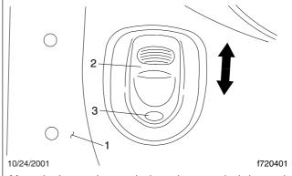
Move the button down to lock, and up to unlock (arrows). The door is unlocked when the red dot shows.
