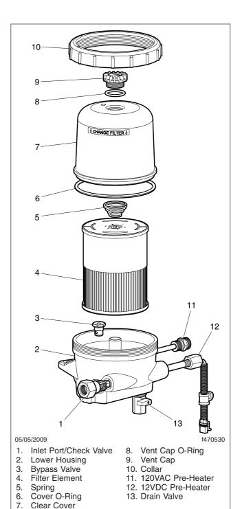
Fig. 21.13, DAVCO Fuel/Water Separator (Fuel Pro 482 shown)
