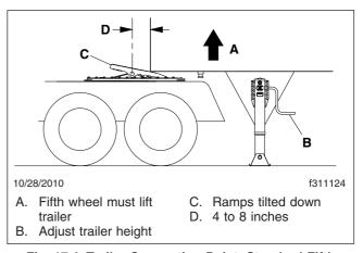
Fig. 17.4, Trailer Connection Point, Standard Fifth Wheel Plate
