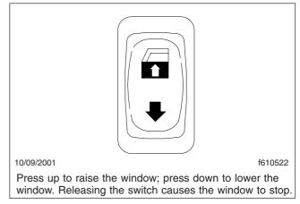
Fig. 8.6, Power Window Switch
