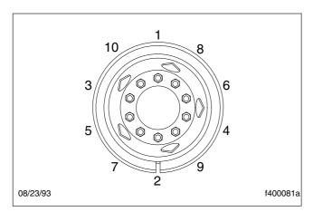
Fig. 21.4, Tightening Pattern, 10-Hole Wheels
