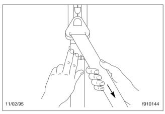
Fig. 6.12, Locking the Komfort Latch
