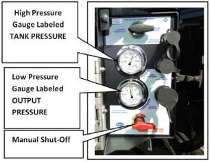
Figure 76. Manual Shut-Off Valve
