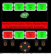
Figure 94. Mutiple Tank Leaks. Maintenance Bypass Required.
