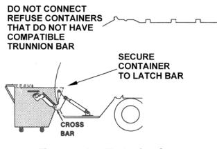
Figure 64. Arm Mechanism Setup
