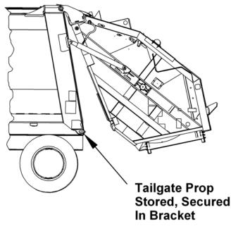
Figure 54. Open Tailgate for Tailgate Props
