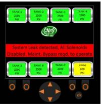
Figure 95. System Leak. Maintenance Bypass Required.
