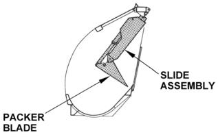
Figure 59. Packer Blade Starting Position
