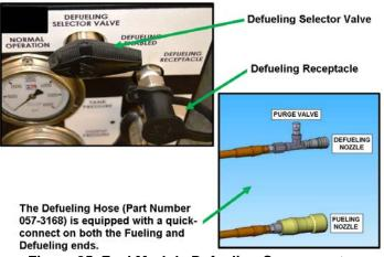
Figure 85. Fuel Module Defueling Components
