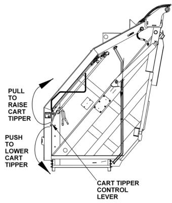
Figure 51. Cart Tipper Control Lever
