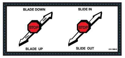
Figure 15. Blade and Slide Controls, PN 212-1969
