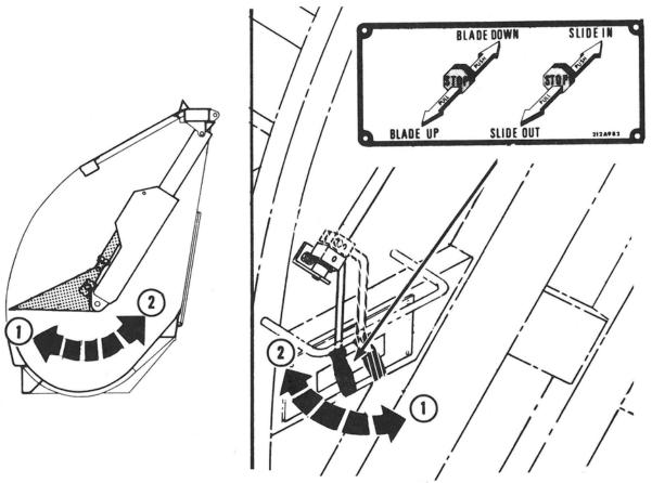
Figure 46. Packer Blade Control Lever
