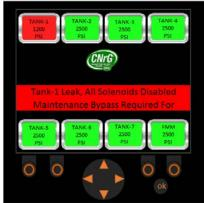
Figure 93. Tank 1 Leak. Maintenance Bypass Required.
