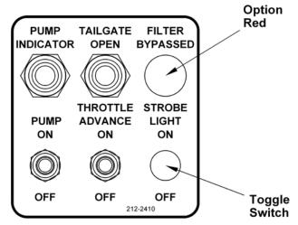
Figure 45. Control Panel Optional Functions
