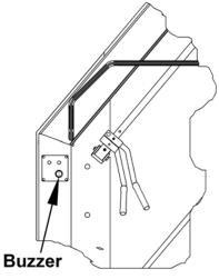
Figure 49. Buzzer Location
