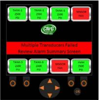
Figure 90. Multiple Pressure Transducer Sensors Unplugged/Faulty
