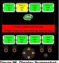
Figure 96. Display Screenshot: Tank 2 Solenoid Failure
