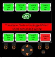
Figure 89. Pressure Transducer Sensor behind FMM Unplugged/Faulty
