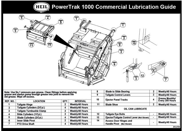
Figure 39. Lubrication Guide, PN 212-2736
