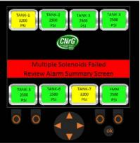
Figure 97. Display Screenshot: Multiple Solenoids Failed
