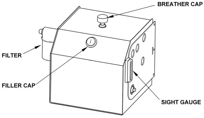
Figure 57. Typical Hydraulic Oil Tank (External Filter)
