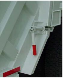
Figure 53. Tailgate Clamps (Turnbuckles)
