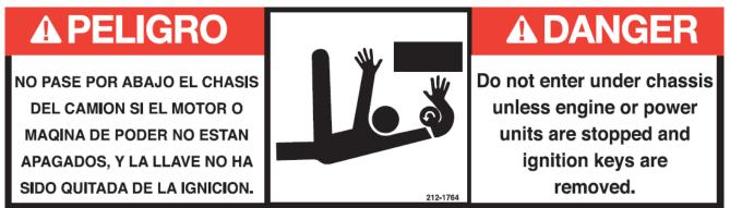
Figure 17. Danger, Under Chassis, Stop Engine, PN 212-1764
