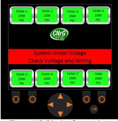
Figure 105. Display Screenshot: System Under Voltage
