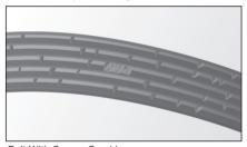
Belt With Severe Cracking
