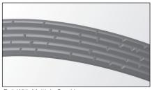
Belt With Multiple Cracking
