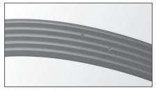
Belt With Minor Cracking
