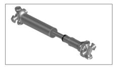
Meritor has developed the Arvin Meritor Extended Lube (MXL) driveshaft series.
