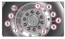
1 1-10 Stud Wheel Nut Tightening Sequence
